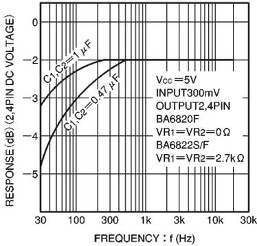
Fig. 10 Frequency characteristics
