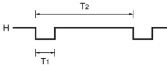
Display switch output duty cycle =  $T_1/T_2$
